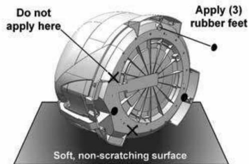
Lay the unit on a soft, non-scratching surface, and apply the (3) rubber feet.
