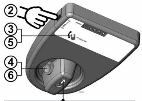
**NOTE:** Arrow on knob indicates which direction antenna is pointing.
